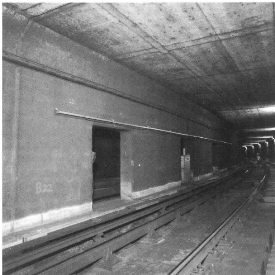
Figure 3. Array of electrolevels installed on subway wall (photo courtesy of Toronto Transit Commission Photographic Services).
